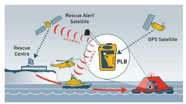
An SPS typically requires an open view of the sky to transmit successfully. Personal Locator Beacons transmit powerful signals at 406 MHz, an internationally recognized distress frequency monitored in the United States by the National Oceanic and Atmospheric Administration and the Air Force Rescue Coordination Center.
